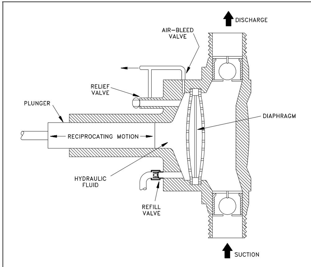
Figure 20 Diaphragm Pump
