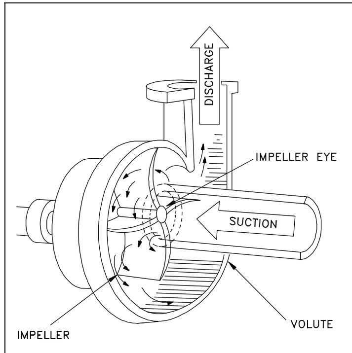
Figure 1 Centrifugal Pump
