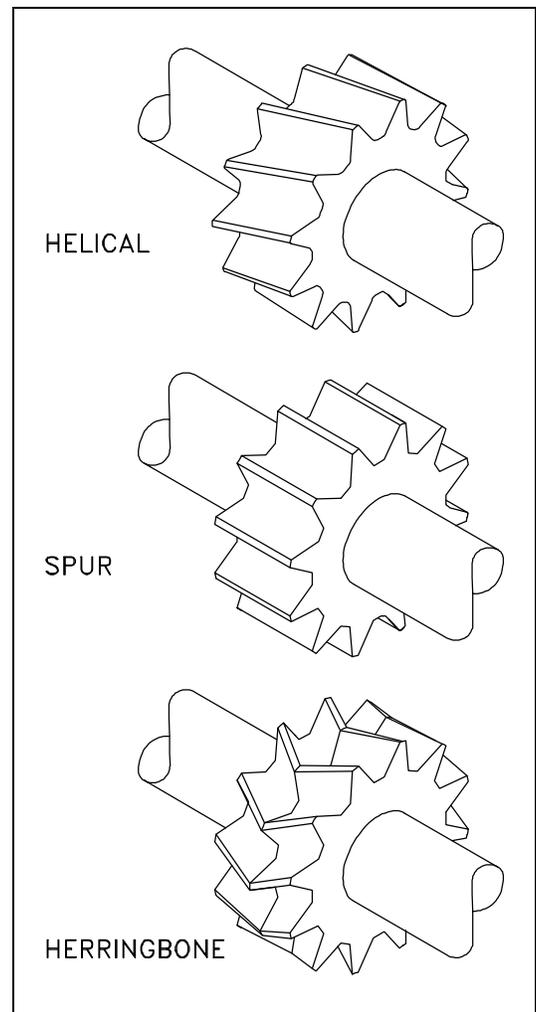
Figure 15 Types of Gears Used In Pumps
